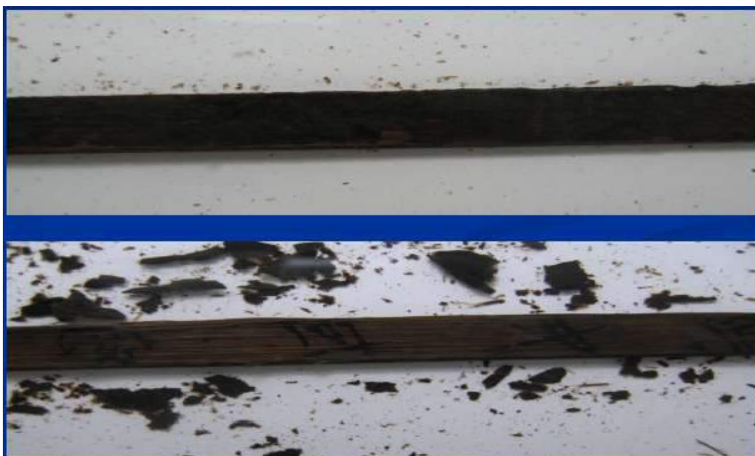
Strips before and after surface material removal.
